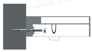
5. Screw a metal nut onto each fixing bolt to secure the basin. Caution: Do not over -tighten, as this may damage the materials.
