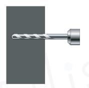
Drill two holes in the required position on the wall using a 14mm masonry drill bit, to a depth of 75mm
