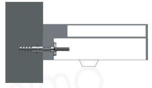
4. Place the basin in position against the wall, iocating the fixing bolts through the holes in the rear of the basin. Push a plastic washer, followed by a metal washer, onto each fixing bolt
